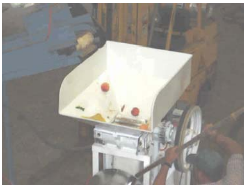
Figure 1. Precrusher breaks up fruit before going into Langsencamp pulper-finisher.
