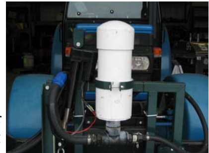
Accumulator reservoir allows a quick gush of spray
