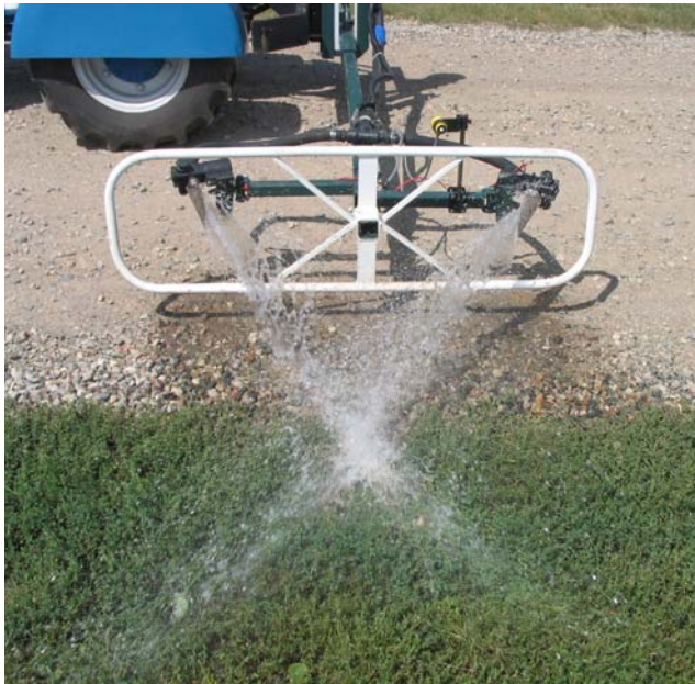
Dual nozzles allow spray to wrap around tree trunk
