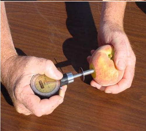
Fruit firmness can be measured with penetrometers available from farm supply businesses. For peaches use a 8 mm diameter tip (5/16” pear tip). Remove a dime to quarter-sized slice of peel, and then use slow uniform force to submerge the tip to the guide mark.
